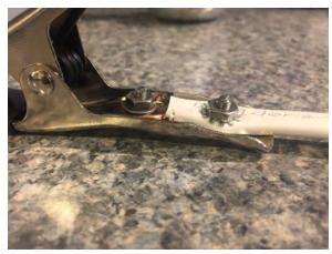
• Gorilla Tape (or shrink wrap) over the exposed bolts nuts and handle
